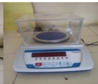
Digital weighing balance (0.1 mg)
