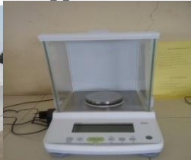
Digital weighing balance-0.01 mg
